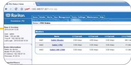
Remote power monitoring, including current (amps), voltage, power (kVA, kW) and energy consumption (kWh)
